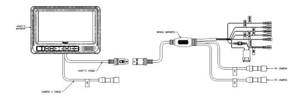
If you need more length for your application, you will need to extend your power/trigger wires and pull additional camera cable up to the monitor's harness or use an additional camera cable to extend the existing cable (p/n **CEC15** -15 ft.).
